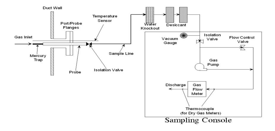
Figure 30B-1. Typical Sorbent Trap Sampling System
